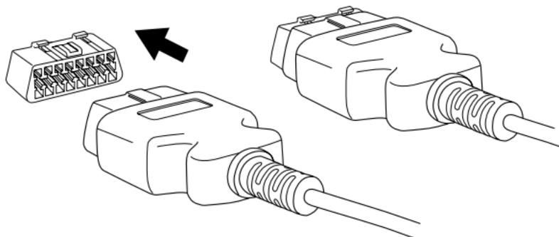
4. Connect the small end of the OBD-II cable to the 10 pin port on the bottom of the Accessport. NOTE: Your Accessport may only have 9 pins. This is by design.
