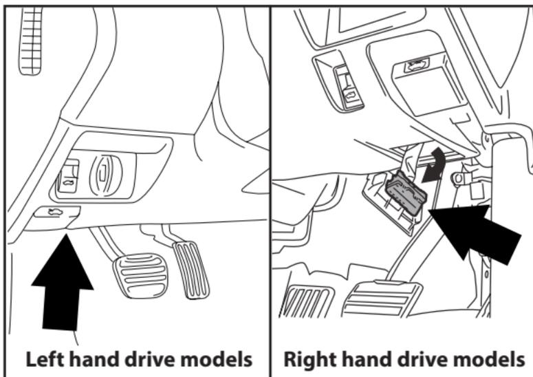
3. Plug the OBD-II cable into the OBD-II port under the dash of vehicle.
