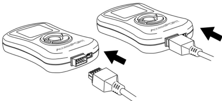
5. Make sure the clasp on the OBD-II cable firmly engages the tab on the 10 pin port.
